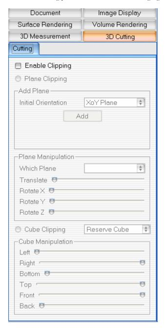
The "Enable Clipping" check box is used to control if the cutting (clipping) is enabled. If you check this option, then the cutting (clipping) is took effect. Otherwise, there is no cutting (clipping) in the volume rendering process. When the cutting (clipping) is turned on, the "Plane Clipping" and "Cube Clipping" radio button is enabled. You can turn "Plane Clipping" on, turn "Cube Clipping" on, or turn both on.
